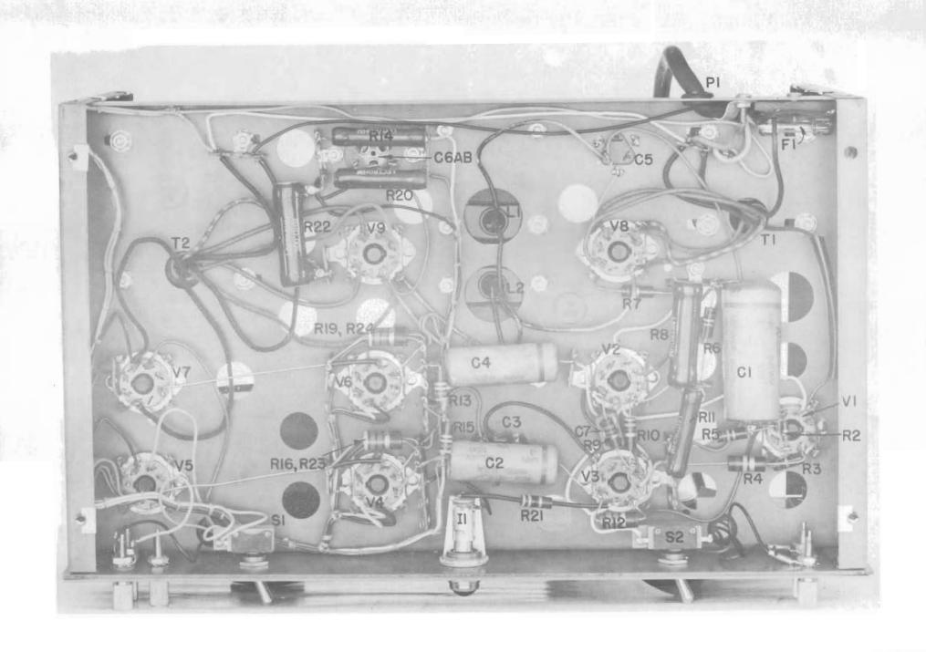
Model 210A Bottom View. Bottom Plate Removed
